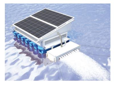
The pressure required for air injection is very less compared to other systems which needs air injection upto the bottom of tanks. Hence current drawn by the micro blower is substantially less making it the most suitable for solar application. All under water parts are plastic with no submersed moving parts. The outside structural material are aluminum and hence also no corrosion problems and maintenance issues.
